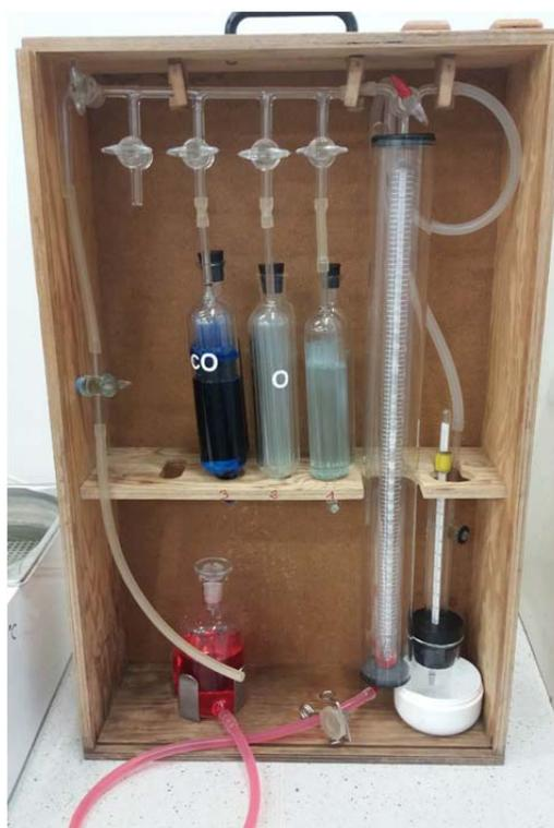
Figure 1: Örsat gas analyzer used during the research
