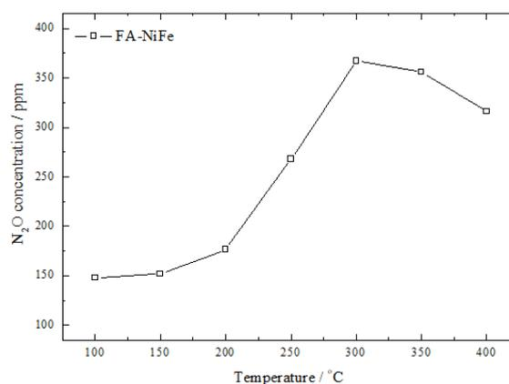
**Chart 4:** N<sub>2</sub>O concentration for fly ash-based catalyst containing nickel and iron (reaction conditions: 800 ppm NO, 800 ppm NH<sub>3</sub>, 3.5 % vol. O<sub>2</sub>, balance He).
