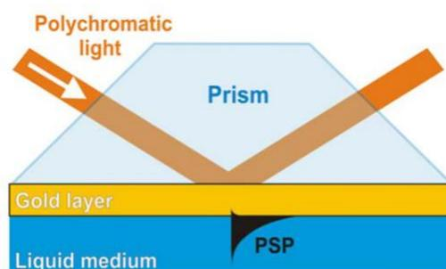
Figure 1. The excitations of PSP's in Kretschmann geometry of an ATR method by a polychromatic light (3)
