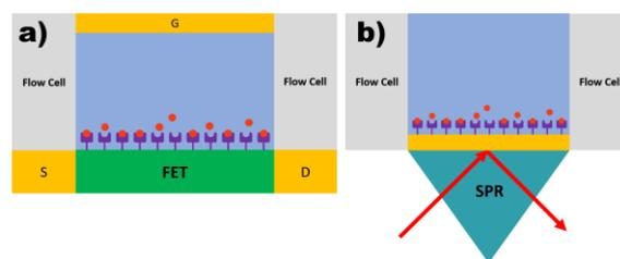
Figure 3. The scheme of the measurement set-up for FET (a) and SPR (b) read-out
