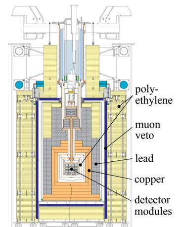
**Figure 1:** The shielding setup of CRESST.
