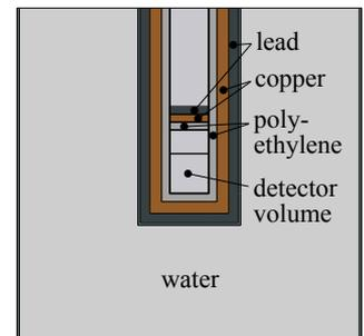
**Figure 3:** Schematic design of the COSINUS shielding.
