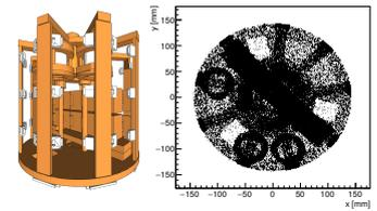
**Figure 2:** left: CRESST detector carousel visualized in Geant4. right: radioactive contamination in its Cu parts
