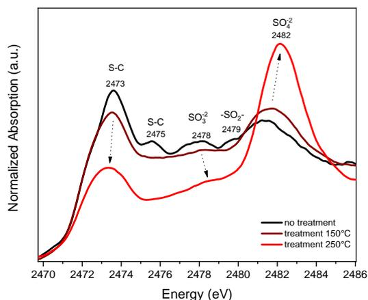
**Figure 2:** XANES spectra at S K-edge of  $Au_{38}/CeO_2$  catalysts fresh and treated at 150°C and 250°C under oxygen atmosphere
