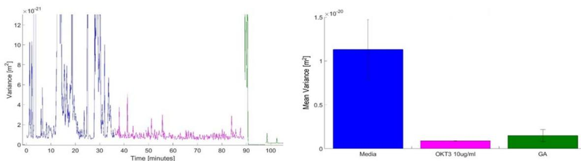
**Figure 2:** Nanomotion oscillation pattern of Jurkat cells exposed to OKT3 antibody that induces T cell activation. It is possible to clearly differentiate between the three states of the T cells: cells in normal media (blue), activated cells (pink) and dead cells (green).
