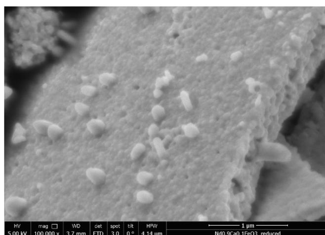
Figure 2: SEM picture of exsolved nanoparticles on  $\text{Nd}_{0.9}\text{Ca}_{0.1}\text{FeO}_3$ .
