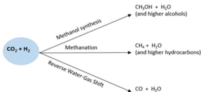
**Figure 1.** Main pathways for the hydrogenation of CO<sub>2</sub>. These pathways are related to temperature, pressure and catalyst.
