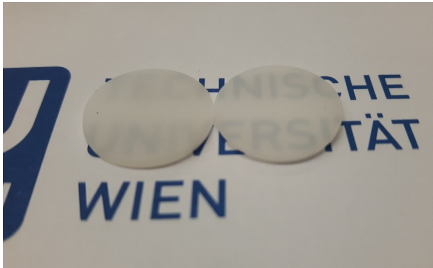
Figure 2: Translucent glass-ceramic test plates produced by LCM
