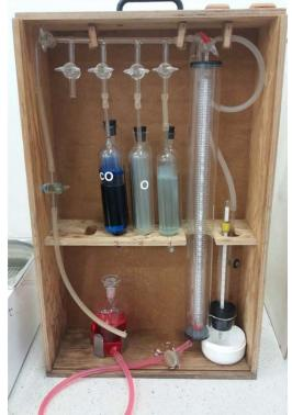
Figure 1: Örsat gas analyzer used during the research
