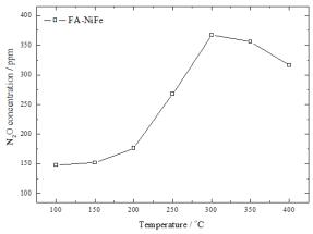
**Chart 1:** NO conversion for fly ash-based catalyst containing nickel and iron (reaction conditions: 800 ppm NO, 800 ppm NH<sub>3</sub>, 3.5 % vol. O<sub>2</sub>, balance He).
