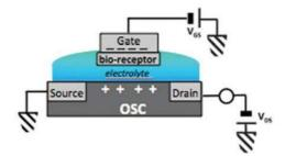
Figure 2. Schematics of an OFET. OSC designates organic semi-conductor (1)
