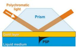
Figure 1. The excitations of PSP's in Kretschmann geometry of an ATR method by a polychromatic light (3)
