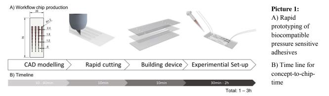
One promising method is to use biocompatible pressure sensitive adhesives to establish microfluidic system for a physiological cell-like environment.
