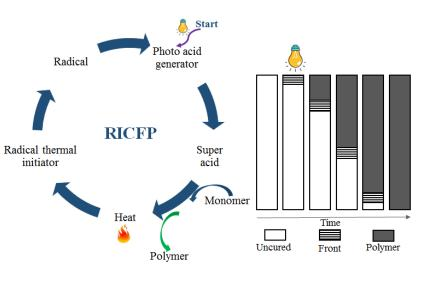
Figure 1: Mechanism and scheme of RICFP
