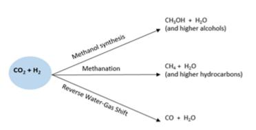
**Figure 1.** Main pathways for the hydrogenation of CO<sub>2</sub>. These pathways are related to temperature, pressure and catalyst.
