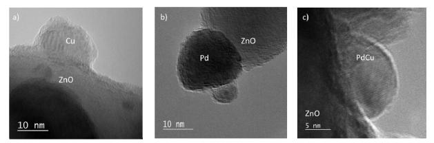
Figure 2. HR-TEM images of Cu/ZnO (a), Pd/ZnO (b) and PdCu/ZnO (c) nanoparticle catalysts
